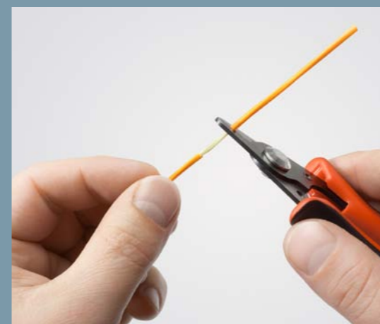
Stripping the FastConnect fiber-optic cable core
